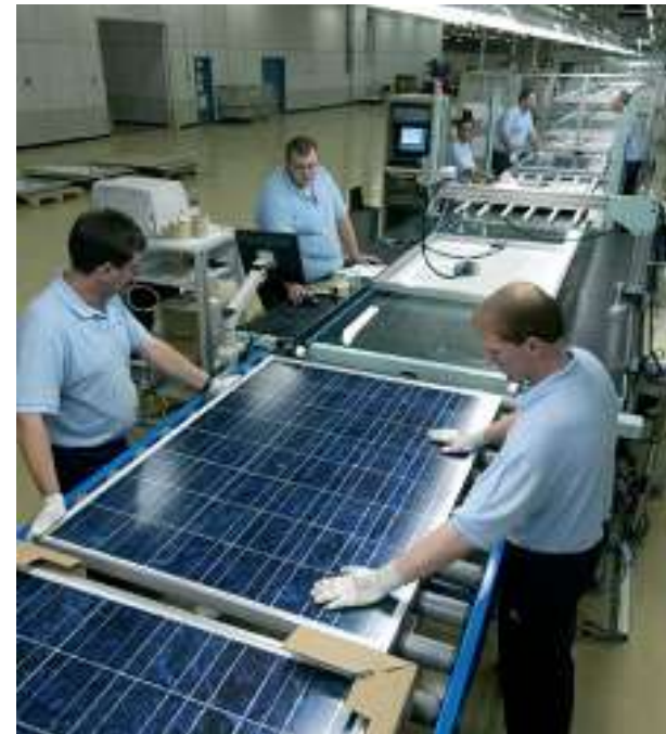
Sharp module factory near Wrexham producing over 300 MW/year
