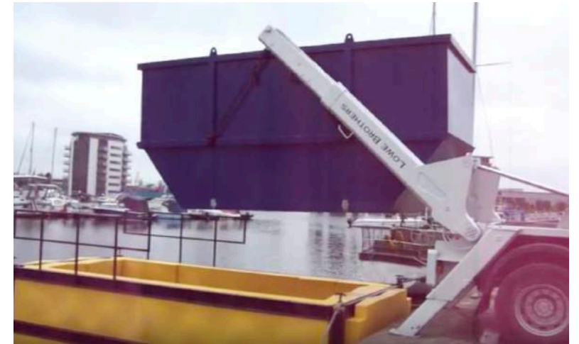
SmartBarge Skip Module Offloading
